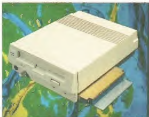
It's not the Chip RAM, but the Agnus chip, in your machine that counts when you install an A570 CD-ROM drive.
